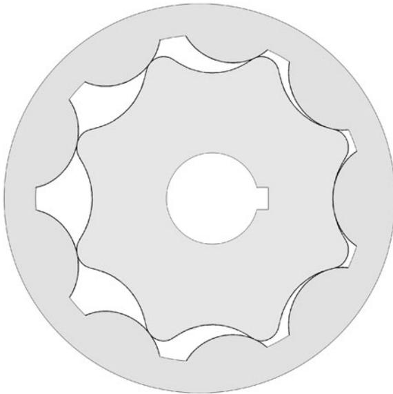
Fig. 1 Elliptical lobe shape pump
