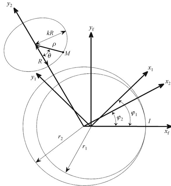
Fig. 2 Coordinate systems and geometrical parameters to generate elliptical lobe shape pumps
