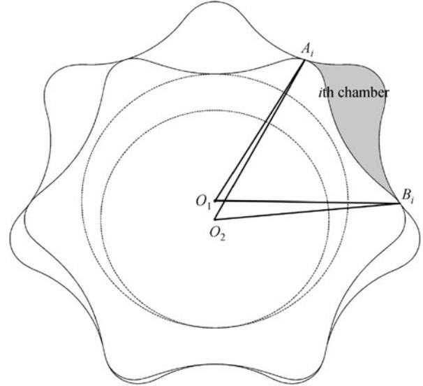
Fig. 3 Corresponding parameters to calculate flow rate for a gerotor pump
