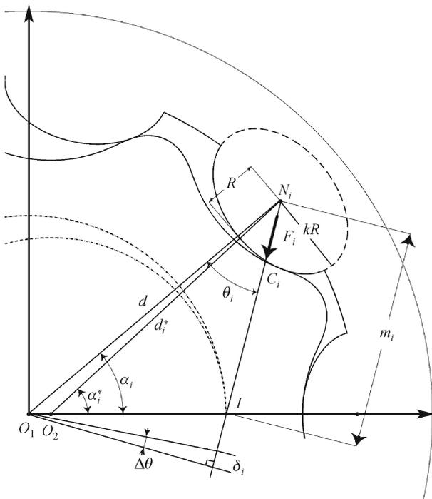
**Fig. 4** Geometrical parameters for sliding velocity and Hertzian contact stress calculation
