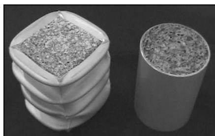
Figure 4. Prototypes of foam-filled tubes developed as crash absorbers. The tubes are aluminum extrusions filled with an aluminum foam. Tube diameter = 65 mm. (Photo courtesy of Cymat.)
