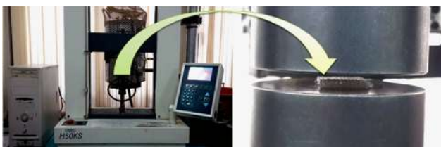
Fig. 3 – View of the performed compression tests setup.
