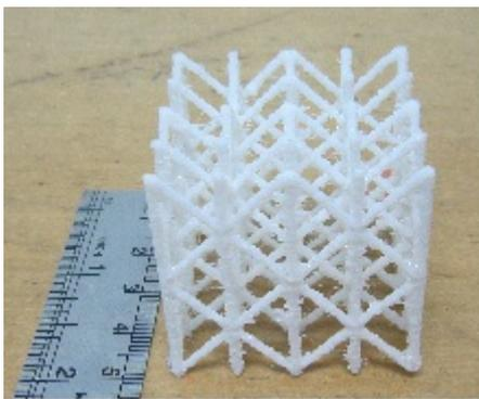
Figure 4: Cellular lattice structures fabricated by the FDM.
