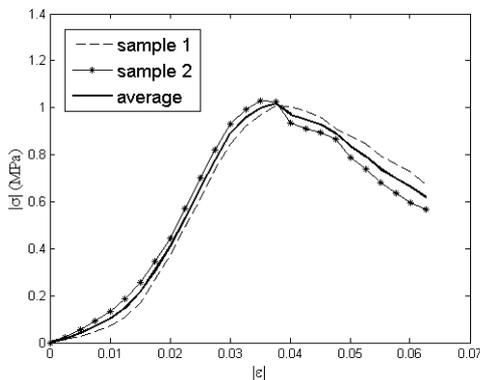
Figure 5: Stress- strain curve of the CLS
