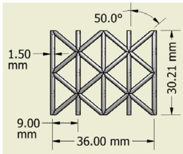
Figure 3: The dimensions of the final version of the cellular lattice structure
