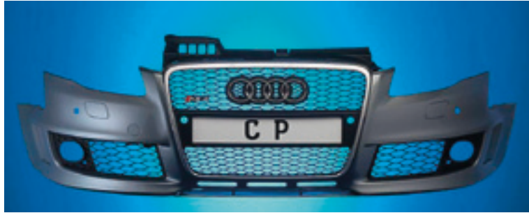
FIGURE 3.9 Modified front spoiler for a special edition car; laser stereolithography, RTV and finishing, spray-painting (Source: CP-GmbH)
