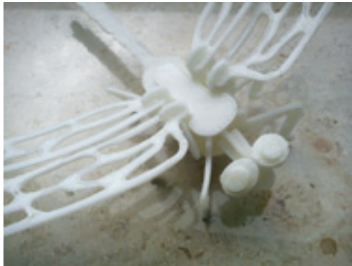
FIGURE 4.25 Self customization: Sculpture of a dragonfly assembled from several parts made from polyamide using the Fabber 1 (source: RP Lab, Aachen University of Applied Sciences)
