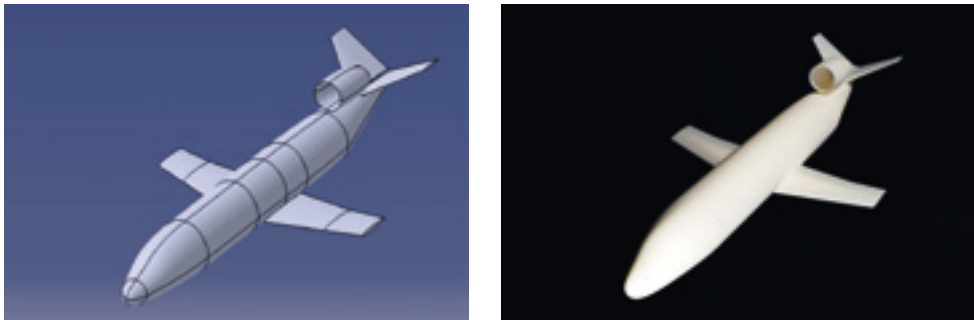
FIGURE 3.43 Single engine airliner concept; rendering (left); AM part, laser sintering of polyimide (right) (Source: Philipp Gebhardt, University of Stuttgart)
