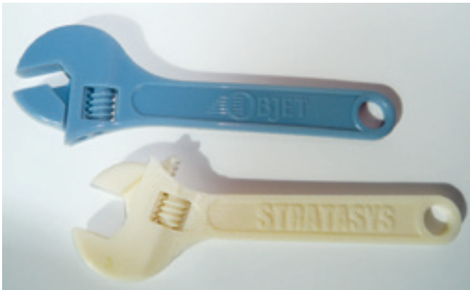
FIGURE 4.5 Scaled wrenches, demonstrators; polymer jetting, acrylate (top); extrusion, FDM, ABS (bottom) (Source: Objet (top), Dimension/Stratasys (bottom))
