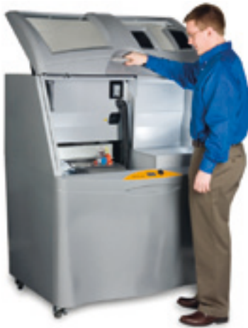
FIGURE 2.17 3D printing. Powder-binder-process; colored parts (top left and right) (Source: RP-Lab, FH Aachen University of Applied Sciences); machine ZPrinter 450 (bottom) (Source: Z-Corporation)
