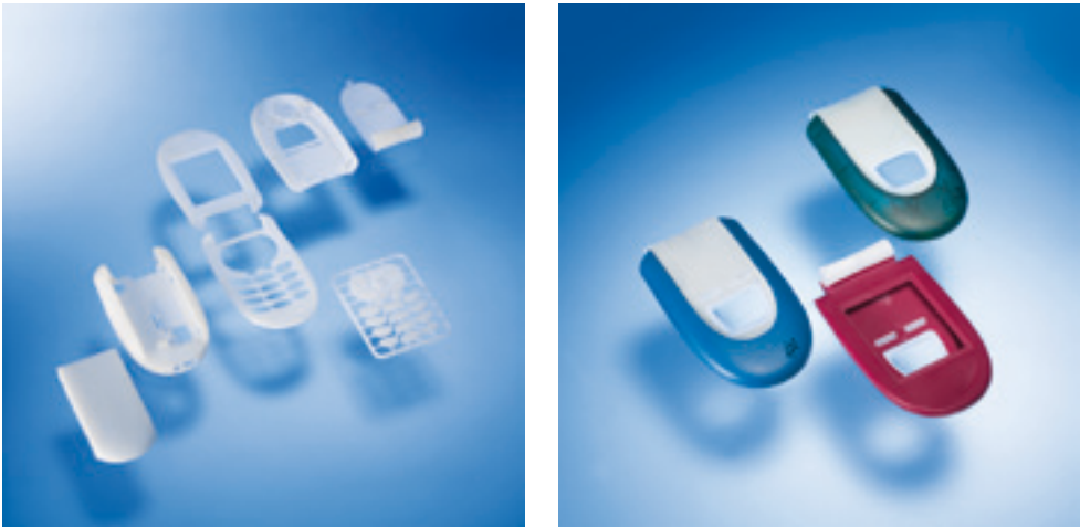
FIGURE 3.13 Mobile phone housing, laser stereolithography masters (left), colored copies by RTV (right) (Source: CP-GmbH)
