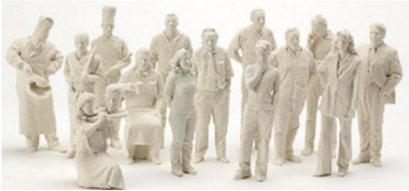
FIGURE 3.24 Body scanning and 3D printing (Z-Corp); plaster-ceramics (Source: Karin Sander/FH-Aachen University of Applied Sciences)
