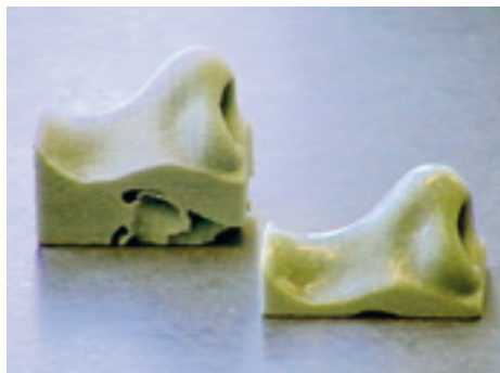
FIGURE 2.18 3D printing. Powder-binder-process; improved surface quality by manual finishing; part as from the machine (left) and after finishing (right) (Source: RP-Lab, FH Aachen University of Applied Sciences)
