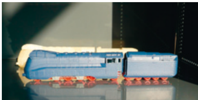
FIGURE 3.22 HO scale (1 : 87) toy train steam engine; stereolithography part after processing (rear); part after post-processing by grinding, decorating, and coloring (front) (Source: CP-GmbH)
