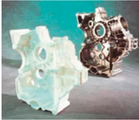
FIGURE 3.31 Lost pattern process; AM master part of a gear box housing made by laser sintering of polystyrene, left; casting, background right (Source: EOS)
