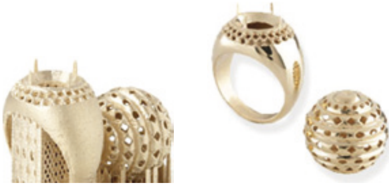
FIGURE 4.18 Customized production; individualization, jewelry direct manufacturing by selected laser melting of gold (Source: Realizer GmbH)
