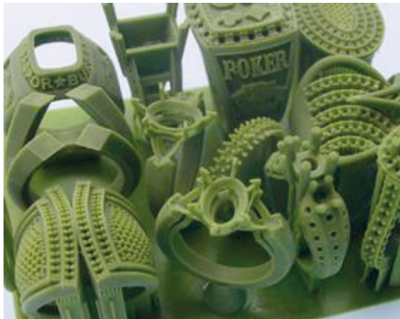
FIGURE 4.17 Customized production; individualization, jewelry masters for investment casting processed in one build (Source: Envisiontec)
