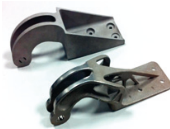
FIGURE 1.12 Direct manufacturing. Aircraft engine cover hinge (bottom) in contrast to the conventionally made one (top). Selective laser melting, SLM, stainless steel (Source: EADS)
