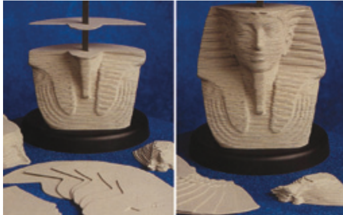
FIGURE 1.1 Principle of layer manufacturing. Contoured layers (left), 3D object made from staggered layers (right) (Source: HASBRO/MB Puzzle)
