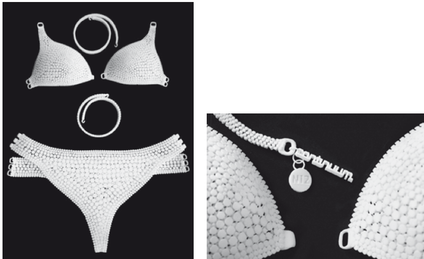
FIGURE 4.13 AM of clothes; “World’s first 3D printed bikini”; laser sintering, polyamide (Source: Continuum Fashion/ Shapeways)
