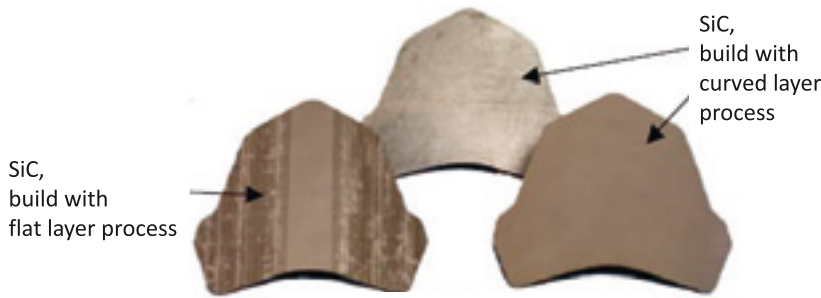
FIGURE 5.5 Layer laminate manufacturing (LLM); reinforced curved parts with integrated SiC fibers /Klo99/
