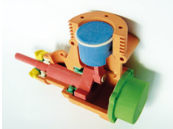
FIGURE 1.6 Solid image or concept model. Cut-away demonstrating part of a combustion engine unit; 3D-printing (Source: Z-Corporation)
