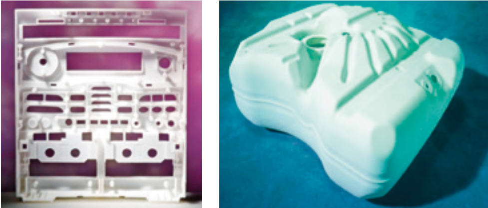
FIGURE 3.6 Dashboard insert; laser sintering, polyamide (left); fuel tank. laser sintering polyamide (right). both: 1 : 1 scale (Source: EOS)
