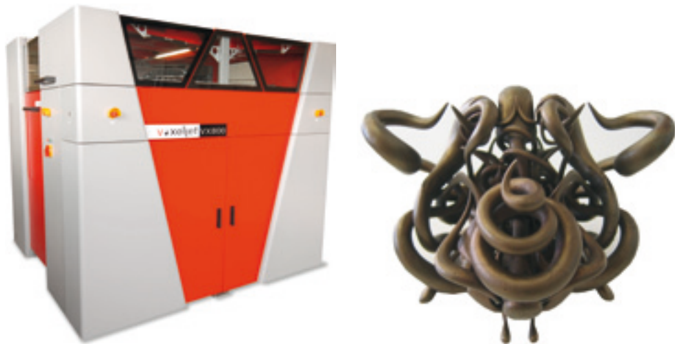
FIGURE 2.20 3D printing. Voxeljet VX800 plastic printer (left), art object “knot” by Josh Harker, finished casting based on a printed master (Source: Voxeljet, www.joshharker.com )
