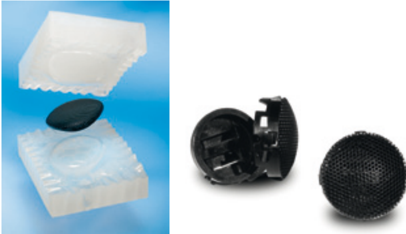
FIGURE 3.7 Speakers, stereolithography master and silicon mold (left), cast part (RTV, right) (Source: CP-GmbH)
