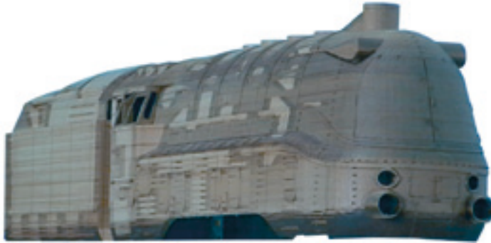
FIGURE 3.21 G-Scale (1 : 22.5) model of a toy train steam engine; laminated object manufacturing (LOM); paper, post-processing by varnishing (Source: CP-GmbH)
