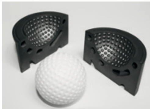
FIGURE 1.15 Steel mold for blow molding. Direct metal laser sintering (Source: EOS/Agie Chamilles)
