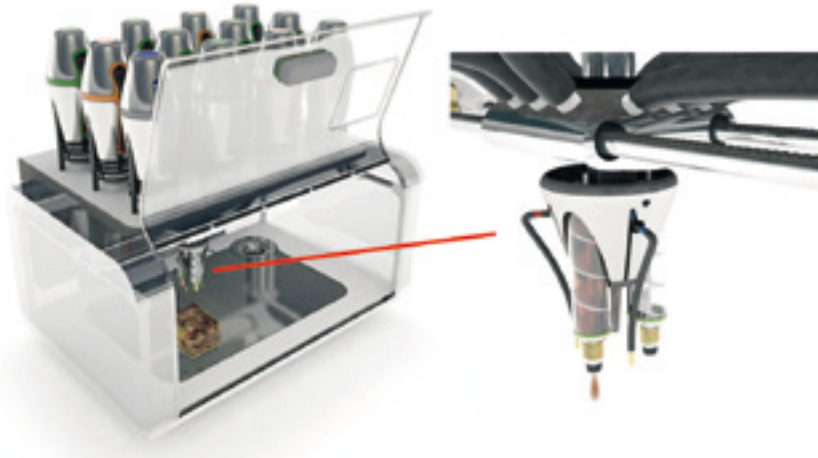
FIGURE 4.15 AM of food; MIT 3D food printer concept “The Cornucopia”; the printer set-up, left; details of the print head, right (Source: Diane Pham/Inhabitat.com)
