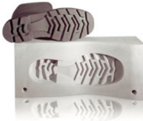
FIGURE 1.17 Prototype tooling; rubber boot sole mold; laser sintering, polyamide (PA) (Source: EOS GmbH)
