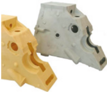
FIGURE 1.30 Indirect manufacturing: Gear box for a racing car; AM master made from PMMA by 3D printing (left), aluminum casting, one-of-a-kind part (right) (Source: Voxeljet)
