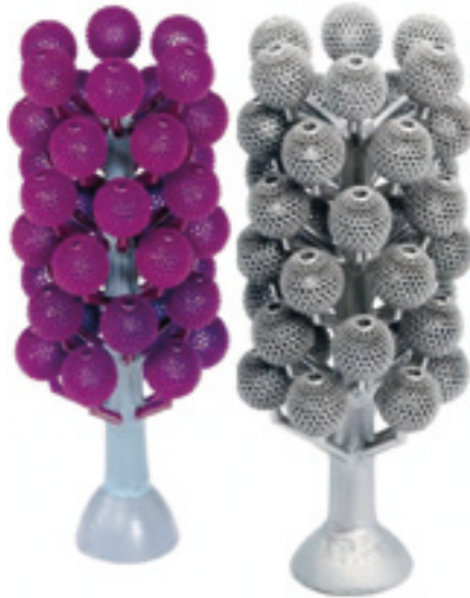
FIGURE 3.30 Investment casting; casting tree made from AM-pattern using wax runners, sprue and gating (left), casting before cleaning (right) (Source: 3D Systems)
