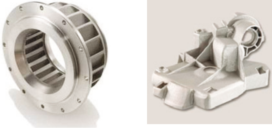
FIGURE 4.4 Guide wheel for an Aero Engine Airplane combustion chamber element (left) Source: EOS/Morris Techn.; hot work steel; base plate (right), aluminum, dimensions 30 \times 100 \times 50 mm (Source: Concept Laser)
