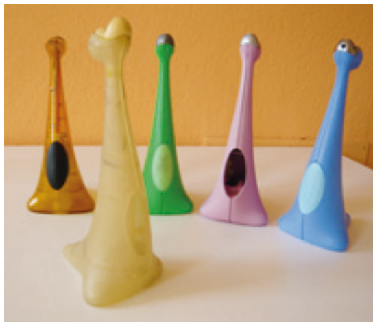
FIGURE 1.22 Indirect prototyping; silicon rubber molding; lighter “Bruce”; AM master, stereolithography; working RTV copies (Source: Alessi/Forum Omega)
