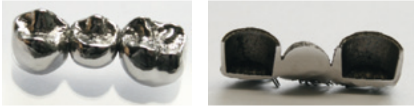
FIGURE 1.11 Direct manufacturing. Three-unit dental bridge (left), cross section (without removal of the supports, right), selective laser melting (SLM); CoCr-alloy (Source: RP Lab, Aachen University of Applied Sciences)
