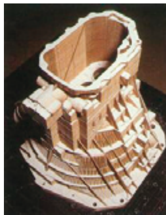
FIGURE 2.22 Layer laminate manufacturing, paper lamination, gear housings (LOM)
