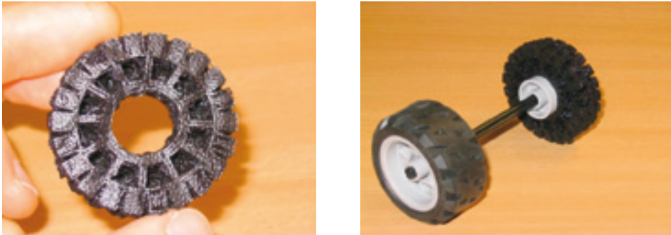
FIGURE 4.24 Self customization; Toy car tire made by Fabber 1, left; mounted on a Lego hub and axis, right background (Source: Fab-at-Home ( www.fabathome.com ))
