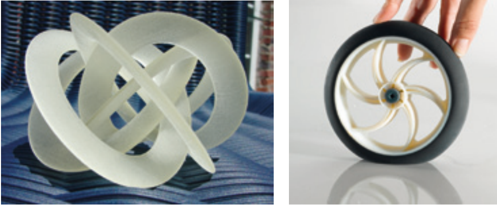
FIGURE 2.7 Polymer jetting (PolyJet, Objet); structure (left); two-material wheel with elastic tire (right) (Source: RP Lab, Aachen University of Applied Sciences, Objet Geometries)
