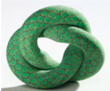
FIGURE 3.42 Decorative element “serpent knot”; colored 3D printing (Source: Z-Corporation)
