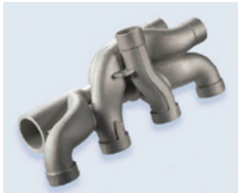
FIGURE 3.10 Exhaust gas manifold of a racing car (Source: Concept Laser/TU Fast e.V.)
