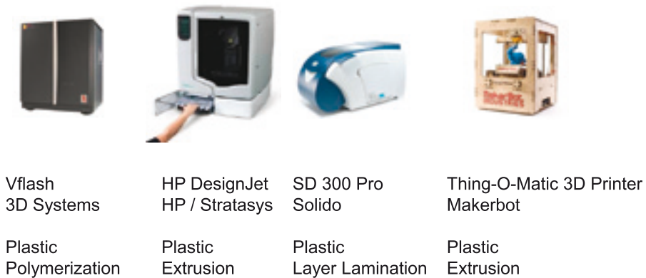
FIGURE 2.27 Layer manufacturing processes: category “fabbers”
