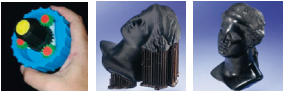
FIGURE 2.16 Fused deposition modeling. Epicyclic gear set assembled from monochromatic FDM parts, made from ABS plastic (left); part with support as manufactured (center); part after removal of the supports and manual polishing (right) (Source: RP-Lab, FH Aachen University of Applied Science (2), Stratasys (1 left))
