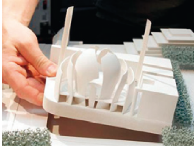
FIGURE 3.37 Architectural model, mosque, laser sintering (Source: Deutschlandwoche, 10/2007)
