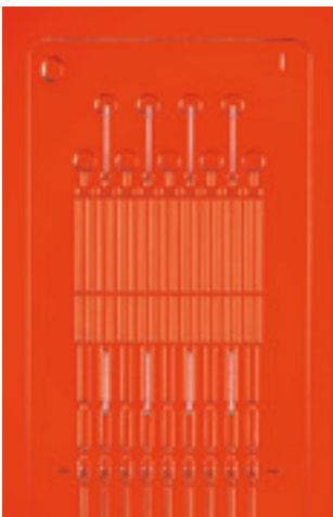
FIGURE 5.10 Microfluidic device, laser stereolithography (Source: 3D Systems)
