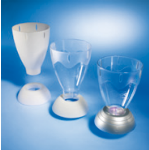
FIGURE 3.14 Cocktail cup, laser stereolithography, RTV and finishing (Source: Pfefferkorn/Toorank/CP-GmbH)
