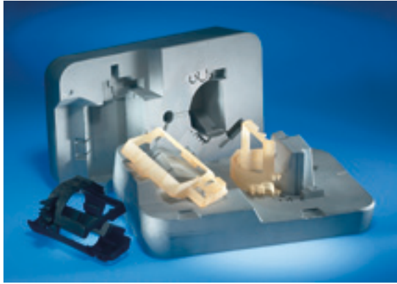
FIGURE 1.26 Indirect tooling. Rigid mold made from aluminum filled epoxy for injection molding of a set of series identical parts (black) based on stereolithography masters (light brown) (Source: Elprotec)
