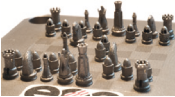
FIGURE 2.13 Micro laser sintering (EOS), demonstrator chess set (Source: EOS GmbH)
