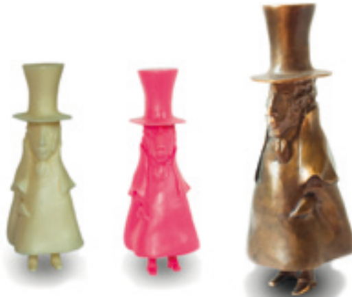
FIGURE 3.25 Sculpture of Alexander Pushkin, made by Alysa Minyukova, NY, using AM and traditional process steps; Laser sintering (left), wax master obtained from RTV (center), final sculpture (right) (Source: Alysa Minyukova, CP-GmbH)
