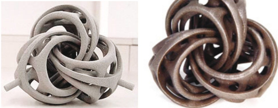
FIGURE 3.23 Art objects; metal 3D printing (Prometal); part after AM production (left) and after post-processing and finishing by surface treatment (Source: Prometal, Bathsheba)
