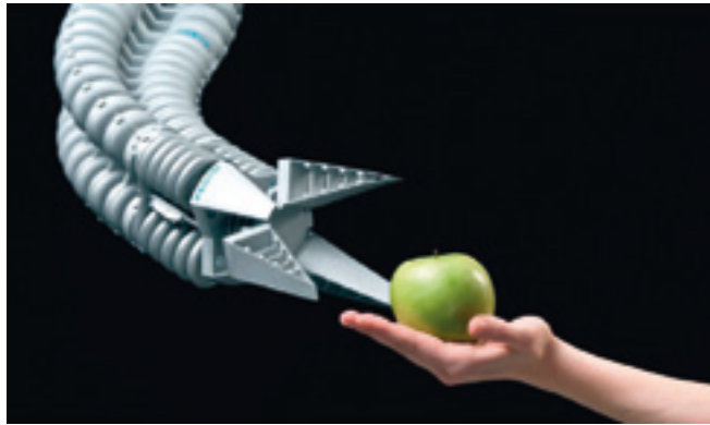
FIGURE 4.10 Bionic handling system resembling an elephant's trunk. Assembled from sintered elements as shown in Fig. 4.9; laser sintering, polyamide (Source: FESTO)
