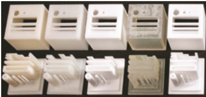
A B C D E Extrusion Polymerization Laser Sintering Polymerization Laser Sintering ABS Epoxy Polyamide Epoxy Polyamide
