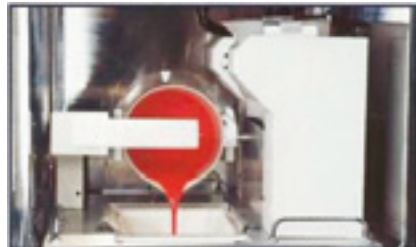
Casting of the PUR Material Solidification by Reaction
