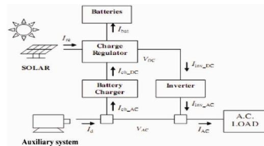
Fig. 1. PV-battery- auxiliary system.
