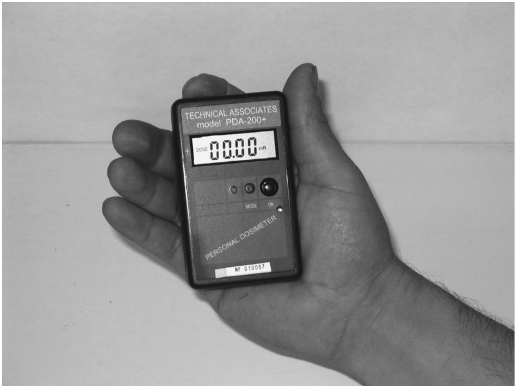
Figure 9-26. Direct-reading electronic dosimeter for personal monitoring. Electronic dosimeters can measure and log beta- and gamma-ray doses from 1 \mu\text{Sv} (0.1 mrem) to about 10 Sv (1000 rems) and contain programmable alarms for cumulative dose and for dose rate. (Courtesy of Technical Associates, Canoga Park, CA.)
