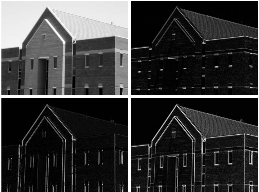
FIGURE 10.18 Same sequence as in Fig. 10.16, but with the original image smoothed using a 5 \times 5 averaging filter prior to edge detection.
