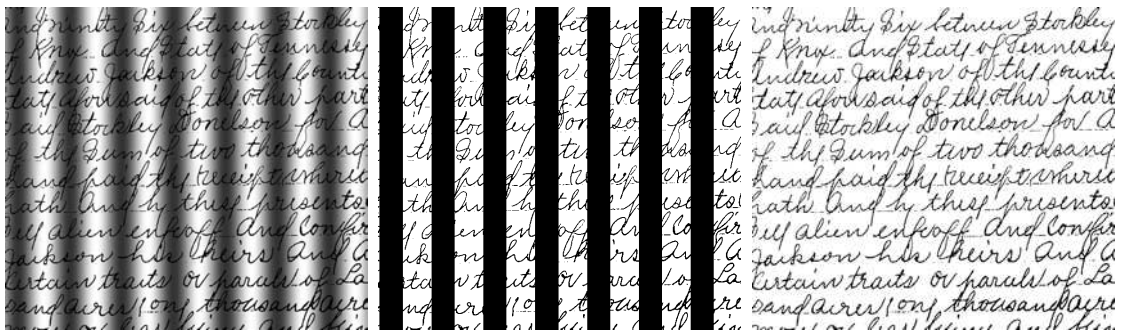
FIGURE 10.50 (a) Text image corrupted by sinusoidal shading. (b) Result of global thresholding using Otsu's method. (c) Result of local thresholding using moving averages.
