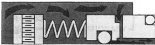
Figure 5. Dynamic o-ring “hang-up.” (Courtesy of Durametallic Corp.)
