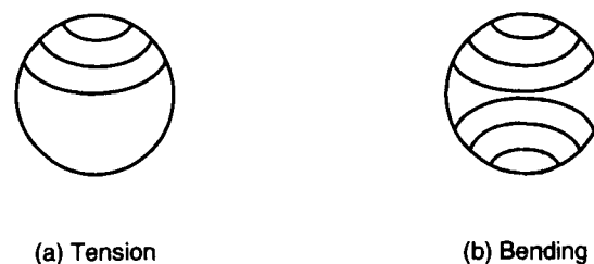
Figure 27. Failure surfaces of round bars subjected to (A) tensile loading and (B) bending.
