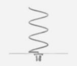
Principle of helical antenna...
