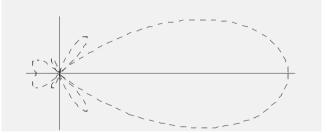
**Fig. 17.4.** Radiation antenna with original parameters n=12 coils and raising angle  $D=10^{\circ}$ , see also Fig. 17.2.
