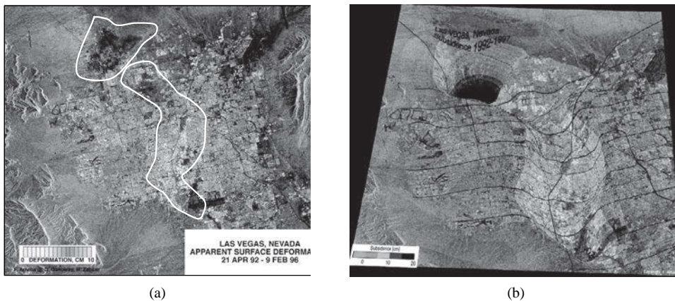
FIGURE 8-27 ■ InSAR-based terrain motion map showing land subsidence in Las Vegas, Nevada, over a nearly four-year period. (a) InSAR-based terrain motion map. Subsidence is significant primarily in the outlined regions, with the subsidence being greatest in the darker region in the upper left quadrant. (b) Three-dimensional visualization of subsidence effects. (Courtesy of the Radar Interferometry Group, Stanford University.)
