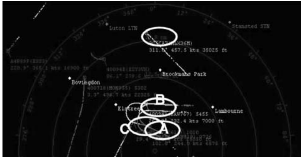
FIGURE 11-14 ■ Air Truth: Mode-S/ ADS-B Virtual Radar Display Corroborating PBR Target Declarations.
