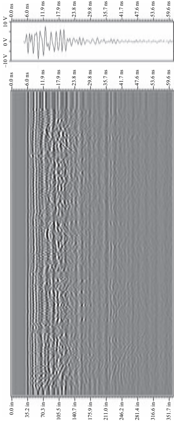
FIGURE 15-62 ■ 1-GHz Ground-Coupled GPR Measured Result, Location 2.
