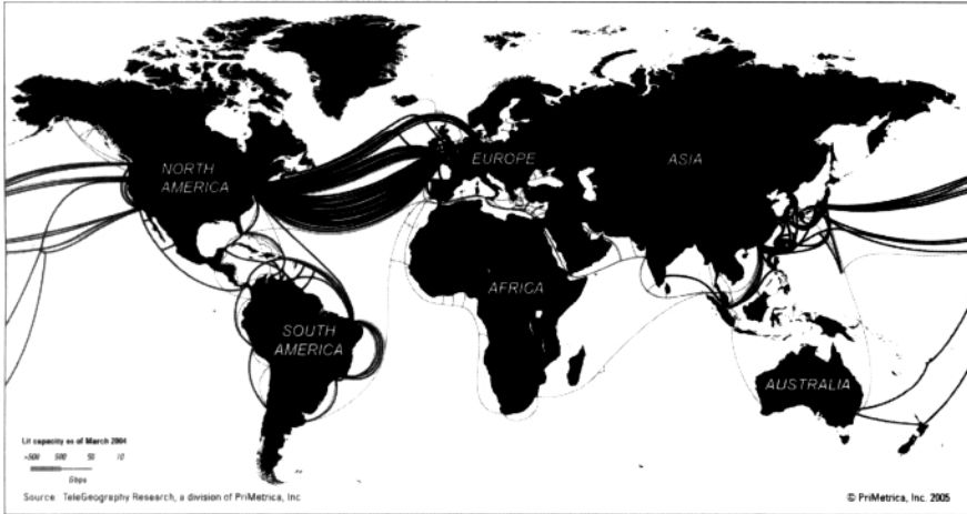
Figure 1.5: International undersea network of fiber-optic communication systems around 2005. (After Ref. [23]; ©2005 IEEE; reprinted with permission.)
