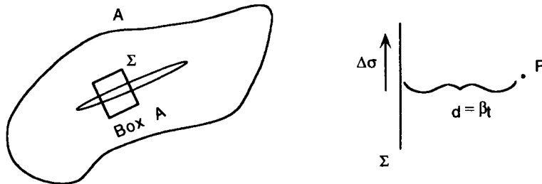
FIGURE 9.17 Geometry of a fault, \Sigma , which cuts a continuous medium. One surface of \Sigma is subjected to a stress that produces a SH wave that travels to a point P .
