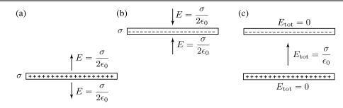
FIGURE 14.2.2: The unbalanced charge at the bottom (a) and top (b) of the slab creates fields of magnitude  $\sigma/(2\epsilon_0)$  oriented as shown. By the linear superposition principle, the total field is given by  $\sigma/\epsilon_0$  within the slab and vanishes elsewhere (c).
