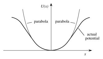
FIGURE 1.4.3: Potential energy function for a centrosymmetric medium.
