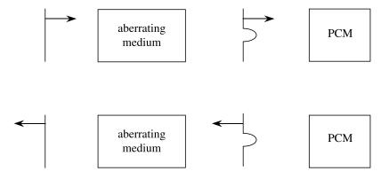
FIGURE 7.2.2: Aberration correction by optical phase conjugation.
