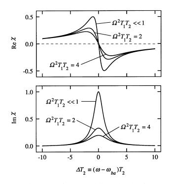
FIGURE 6.3.1: Real and imaginary parts of the susceptibility  $\chi$  (in units of  $\alpha_0 c/\omega_{ba}$ ) plotted as functions of the optical frequency  $\omega$  for several values of the saturation parameter  $\Omega^2 T_1 T_2$ .
