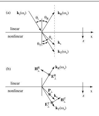
FIGURE 2.11.2: (a) Geometry showing the creation of a transmitted and reflected second-harmonic wave at the surface of a second-order nonlinear optical material. (b) Definition of the electric and magnetic field vectors for the case in which  $\mathbf{P}$  is perpendicular to the plane of incidence.
