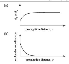
FIGURE 10.4.2: Nature of Raman amplification for the case of perfect phase matching ( $\Delta k = 0$ ).
