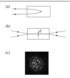
FIGURE 7.1.1: Schematic illustration of three self-action effects: (a) self-focusing of light, (b) selftrapping of light, and (c) laser beam breakup, showing the transverse distribution of intensity of a beam that has broken up into many filaments.
