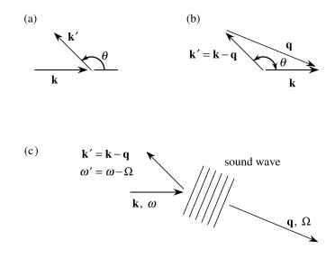
FIGURE 8.3.1: Illustration of Stokes Brillouin scattering.
