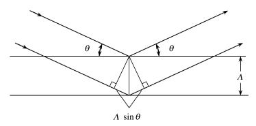
FIGURE 8.4.2: The Bragg condition for acoustooptic scattering.
