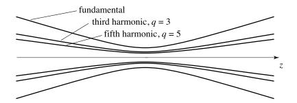
FIGURE 2.10.2: Variation of the beam parameter w(z) in the focal region for the fundamental and thirdand fifth-harmonic beams. All three fields have the same confocal parameter b, although the beam waist radius  $w_0$  and far field diffraction angle scale as  $q^{-1/2}$ .
