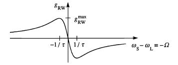
FIGURE 10.6.2: Frequency dependence of the gain factor for stimulated Rayleigh-wing scattering.
