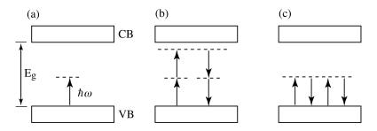
FIGURE 4.6.4: (a) For  $\hbar\omega < E_g$ , the nonlinear response involves virtual transitions. Under many circumstances, virtual two-photon processes (b) make a larger contribution to the nonlinear response than do one-photon processes (c).
