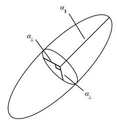
FIGURE 10.6.1: Illustration of the polarizabilities of an anisotropic molecule for the case  $\alpha_{\parallel} > \alpha_{\perp}$ .
