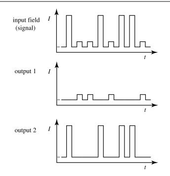
FIGURE 7.3.7: Illustration of the use of the device of Fig. 7.3.6 (without a control field) as a pulse sorter. The weaker pulses are routed to output 1, and the stronger pulses are routed to output 2.
