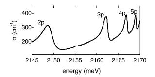
FIGURE 4.6.2: Absorption spectrum of  $Cu_2O$  at a temperature of 4.2 K. The spectral features result from transitions from the top of the valence band to the exciton level labeled in the figure. (After Tayagaki et al., 2005.)
