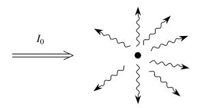
FIGURE 8.1.4: Scattering of light by a molecule.
