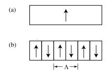
FIGURE 2.4.1: Schematic representations of a second-order nonlinear optical material in the form of (a) a homogeneous single crystal and (b) a periodically poled material in which the positive c axis alternates in orientation with period  $\Lambda$ .
