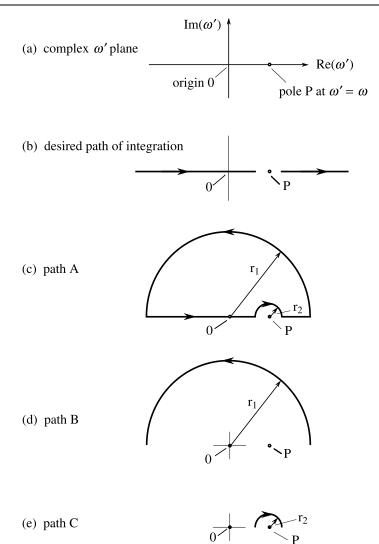
FIGURE 1.7.1: Diagrams used in the contour integration of Eq. (1.7.3). (a) shows the complex  $\omega'$  plane, (b) shows the desired path of integration, and (c), (d), and (e) show paths over which the integral can be evaluated using the techniques of contour integration. In performing the integration the limits  $r_1 \rightarrow \infty$  and  $r_2 \rightarrow 0$  are taken.
