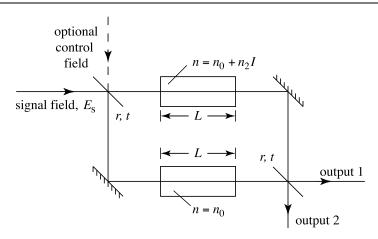
FIGURE 7.3.6: Configuration of an all-optical switch in the form of a Mach–Zehnder interferometer containing a nonlinear element. The input signal field is routed to either output 1 or 2 depending on its intensity and/or on the intensity of the control field.
