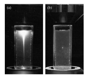
FIGURE 12.5.2: Fluorescence from a dye solution (20  $\mu$ M solution of fluorescence in water) under (a) one-photon excitation and (b) two-photon excitation. Note that under two-photon excitation, fluorescence is excited only at the focal spot of the incident laser beam. Photographs courtesy of W. Webb.
