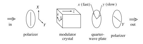
FIGURE 11.3.3: Construction of a voltage-controllable intensity modulator.
