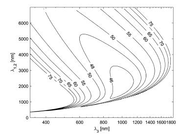
FIGURE 2.3.4: Phase matching curves for type-I collinear phase matching in lithium niobate. Here  $\lambda_3$  is the wavelength of the wave with the highest frequency, and the low frequency waves have wavelengths  $\lambda_1$  and  $\lambda_2$ . The number that labels each curve is the phase matching angle in degrees.
