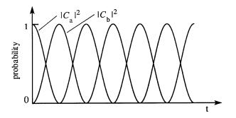
FIGURE 6.5.1: Rabi oscillations of the populations in the ground  $(|C_a|^2)$  and excited  $(|C_b|^2)$  states for the case of exact resonance ( $\Delta = 0$ ).
