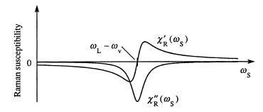
FIGURE 10.3.3: Resonance structure of the Raman susceptibility.
