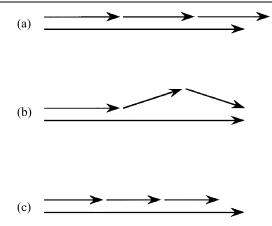
FIGURE 2.10.4: Illustration of why a positive value of  $\Delta k$  is desirable in harmonic generation with focused laser beams. (a) Wavevector diagram for third-harmonic generation with  $\Delta k$  positive. Even though the process is phase mismatched, the fundamental beam contains an angular spread of wavevectors and the phase-matched process illustrated in (b) can occur with high efficiency. (c) Conversely, for  $\Delta k$  negative, efficient harmonic generation cannot occur.
