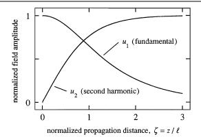
FIGURE 2.7.3: Spatial variations of the fundamental and second-harmonic field amplitudes for the case of perfect phase matching and the boundary condition  $u_2(0) = 0$ .
