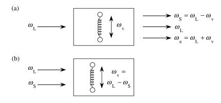
FIGURE 10.3.2: Stimulated Raman scattering. (a) A laser beam at frequency  $\omega_L$  scatters off a molecule vibrating at frequency  $\omega_v$  to generate light at the Stokes frequency  $\omega_S$  and the anti-Stokes frequency  $\omega_a$ . (b) Light beams at frequencies  $\omega_L$  and  $\omega_S$  illuminate a molecule. The beat note between these two frequencies drive a molecular vibration at frequency  $\omega_v = \omega_L - \omega_S$ .
