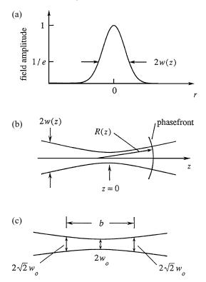
FIGURE 2.10.1: (a) Field amplitude distribution of a Gaussian laser beam. (b) Variation of the beam radius w and wavefront radius of curvature R with position z. (c) Relation between the beam waist radius and the confocal parameter b.
