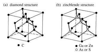
FIGURE 1.5.4: Illustration of (a) the diamond structure and (b) the zincblende structure. Both possess a cubic lattice and thus cannot display birefringence, but the carbon structure is centrosymmetric, whereas the zincblende structure is noncentrosymmetric.
