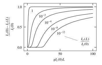
FIGURE 9.3.3: Intensity transfer characteristics of an SBS amplifier.
