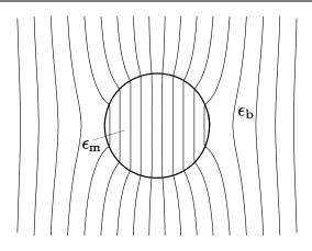
FIGURE 14.6.1: Electric field distribution in the neighborhood of a polarizable sphere placed in an otherwise uniform electric field. The situation  $\epsilon_m = 2$  and  $\epsilon_b = 1$  is shown. Note that the electric field is drawn in towards the region of the sphere.
