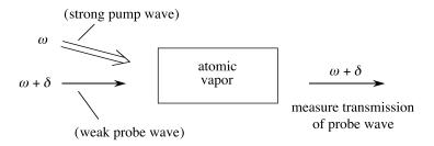
FIGURE 6.6.1: Saturation spectroscopy setup.
