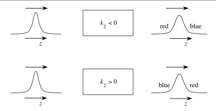
FIGURE 7.5.3: Pulse spreading resulting from group velocity dispersion.
