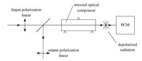
FIGURE 7.2.7: Polarization properties of phase conjugation.
