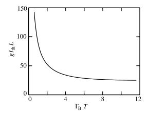
FIGURE 9.3.6: Dependence of the SBS threshold intensity  $I_{\rm th}$  on the laser pulse duration T.
