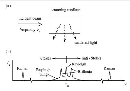
FIGURE 8.1.1: Spontaneous light scattering. (a) Experimental setup. (b) Typical observed spectrum.
