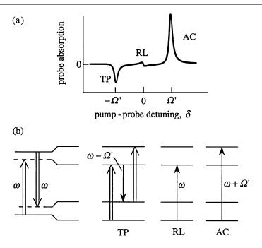
FIGURE 6.6.4: (a) Absorption spectrum of a probe wave in the presence of a strong pump wave for the case  $\Delta T_2 = -3$ ,  $\Omega T_2 = 8$ , and  $T_2/T_1 = 2$ . (b) Each of the features in the spectrum shown in part (a) is identified by the corresponding transition between dressed states of the atom. TP denotes the three-photon resonance, RL denotes the Rayleigh resonance, and AC denotes the ac-Stark-shifted atomic resonance.
