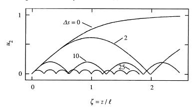
FIGURE 2.7.4: Effect of wavevector mismatch on the efficiency of second-harmonic generation.
