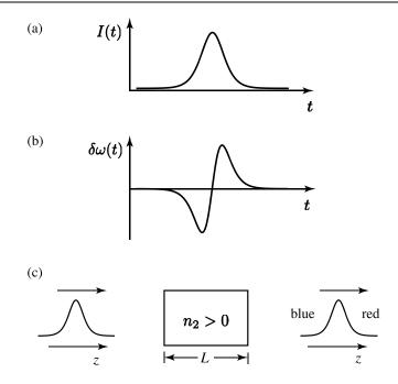
FIGURE 7.5.1: (a) Time dependence of the incident pulse. (b) Change in instantaneous frequency of the transmitted pulse. (c) Laboratory arrangement to observe self-phase modulation.
