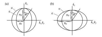
FIGURE 2.12.2: Refractive index surfaces for (a) negative and (b) positive uniaxial crystals. These curves show how the refractive index varies as a function of the propagation direction (**k**-vector direction) within the crystal.
