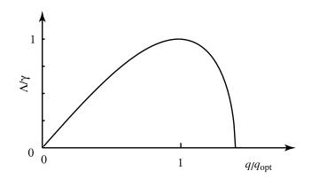
FIGURE 7.1.7: Variation of the gain coefficient  $\Lambda$  of the forward four-wave mixing process that leads to laser-beam breakup with the transverse wavevector magnitude q.
