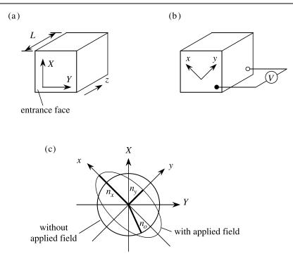
FIGURE 11.3.1: The electrooptic effect in KDP. (a) Principal axes in the absence of an applied field. (b) Principal axes in the presence of an applied field. (c) The intersection of the index ellipsoid with the plane z = Z = 0.
