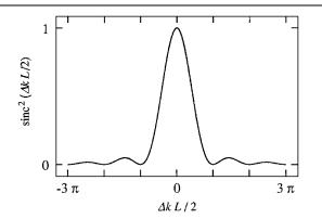
FIGURE 2.2.2: Effects of wavevector mismatch on the efficiency of sum-frequency generation.
