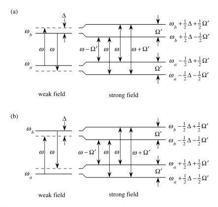
FIGURE 6.5.3: Frequency spectrum of the atomic wavefunction given by Eq. (6.5.4) (with  $C_a(t)$  and  $C_b(t)$  given by Eqs. (6.5.28) and (6.5.29)) for the case of (a) positive detuning ( $\Delta > 0$ ) and (b) negative detuning ( $\Delta < 0$ ).
