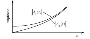
FIGURE 2.8.2: Spatial evolution of  $A_1$  and  $A_2$  for difference-frequency generation for the case  $\Delta k = 0$  in the constant-pump approximation.
