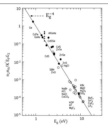
FIGURE 4.6.6: Comparison of the predictions (solid line) of the model of Sheik-Bahae et al. (1991) with measured values (data points) of the nonlinear refraction parameter  $n_2$  for a variety of materials.
