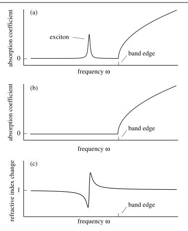
FIGURE 4.6.3: Schematic low-temperature absorption spectrum of a semiconductor in the absence (a) and in the presence (b) of an appreciable number of optically excited conduction band electrons. (c) The modification of the refractive index associated with the optically induced change in absorption coefficient.
