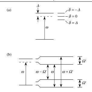
FIGURE 6.6.3: Resonances in the response of a two-level atom to pump and probe fields, as given by the function  $D(\delta)$ , (a) in the limit  $\Omega^2 \rightarrow 0$ , and (b) in the general case.
