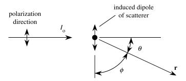
FIGURE 8.2.1: Geometry of light scattering from an individual molecule.
