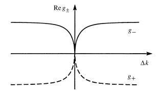
FIGURE 10.4.1: Dependence of the coupled gain on the wavevector mismatch.
