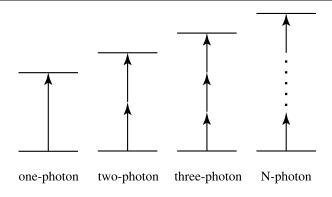
FIGURE 12.5.1: Several examples of multiphoton absorption processes.
