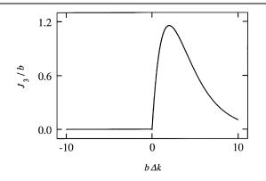
FIGURE 2.10.3: Dependence of the phase-matching factor  $J_3$  for third-harmonic generation on the normalized confocal parameter  $b\Delta k$ , in the tight-focusing limit.
