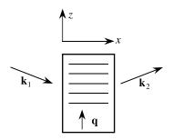
FIGURE 8.4.4: Geometry of a Bragg-type acoustooptic modulator.
