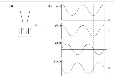
FIGURE 11.4.1: Origin of the photorefractive effect. (a) Two light beams form an interference pattern within a photorefractive crystal. (b) The resulting distributions of intensity I(x), charge density  $\rho(x)$ , induced static field amplitude E(x), and induced refractive index change  $\Delta n(x)$  are illustrated.
