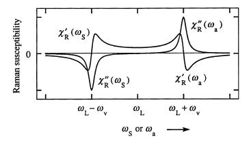
FIGURE 10.3.4: Relation between Stokes and anti-Stokes Raman susceptibilities.
