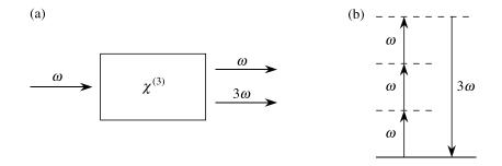
FIGURE 1.2.5: Third-harmonic generation. (a) Geometry of the interaction. (b) Energy-level description.
