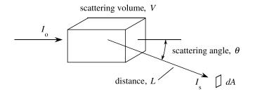
FIGURE 8.1.3: Quantities used to define the scattering coefficient.
