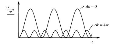
FIGURE 2.6.3: Spatial variation of the sum-frequency wave in the undepleted-pump approximation.
