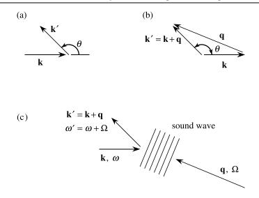
FIGURE 8.3.2: Illustration of anti-Stokes Brillouin scattering.
