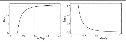
FIGURE 14.3.1: The frequency dependence of the real and imaginary parts of the dielectric permittivity  $\epsilon(\omega)$  according to the Drude model.
