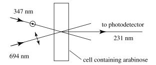
FIGURE 5.5.2: Experimental setup to observe sum-frequency generation in an isotropic, chiral medium.
