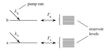
FIGURE 6.2.3: Relaxation processes for the open two-level atom.
