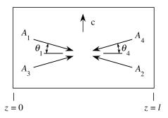
FIGURE 11.7.1: Geometry of four-wave mixing in a photorefractive material.
