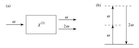
FIGURE 1.2.1: (a) Geometry of second-harmonic generation. (b) Energy-level diagram describing second-harmonic generation.
