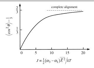
FIGURE 4.4.3: Variation of the quantity  $(\langle \cos^2 \theta \rangle - \frac{1}{3})$ , which is proportional to the nonlinear change in refractive index  $\delta n$ , with the intensity parameter *J*. Note that for  $J \leq 5$ ,  $\delta n$  increases nearly linearly with *J*.
