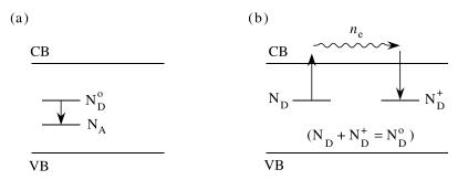
FIGURE 11.5.1: Energy levels and populations used in the model of Kukhtarev et al. to describe the photorefractive effect.
