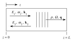
FIGURE 9.3.1: Schematic representation of the stimulated Brillouin scattering process.
