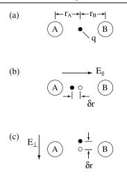
FIGURE 5.4.1: The bond-charge model applied to a chemical bond between constituents A and B. Parts (b) and (c) show how the charge moves in response to applied electric fields.
