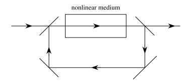
FIGURE 7.3.2: Bistable optical device in the form of a traveling wave interferometer containing a nonlinear medium.
