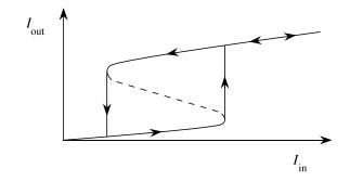
FIGURE 1.2.9: Typical input-versus-output characteristics of a bistable optical device.
