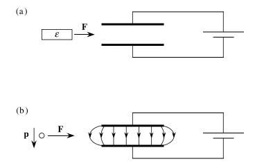
FIGURE 9.2.1: Origin of electrostriction: (a) a dielectric slab placed near a parallel-plate capacitor will be drawn into the region between the capacitor plates. (b) A molecule placed in the fringing field of a parallel-plate capacitor will develop a dipole moment  $\mathbf{p}$  and will thus experience a force in the direction of increasing field strength.
