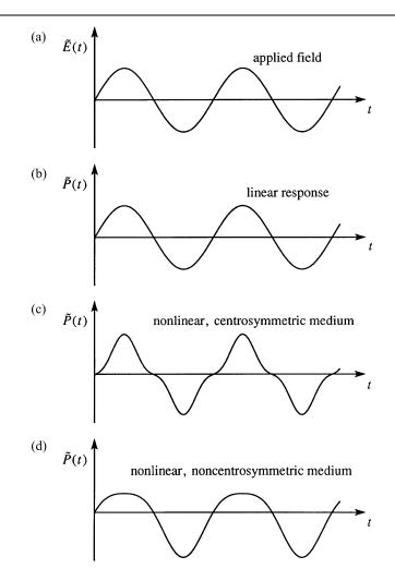
FIGURE 1.5.2: Waveforms associated with the atomic response.
