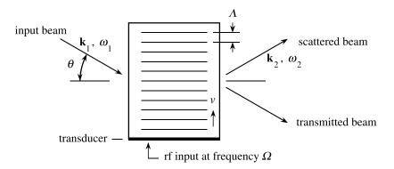
FIGURE 8.4.1: Bragg-type acoustooptic modulator.
