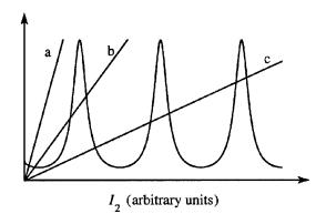
FIGURE 7.3.5: Graphical solution to Eq. (7.3.19). The oscillatory curve represents the right-hand side of this equation, and the straight lines labeled a through c represent the left-hand side for increasing values of the input intensity  $I_1$ .
