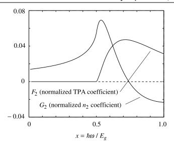
FIGURE 4.6.5: Variation of the nonlinear refraction coefficient  $n_2$  and the two-photon-absorption coefficient with photon energy  $\hbar\omega$  according to the model of Sheik-Bahae et al. (1990).
