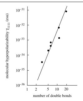
FIGURE 5.3.2: Measured dependence of the value of the hyperpolarizability  $\gamma_{1111}$  on the number of double bonds in the molecule. The data are from Hermann and Ducuing (1974) and the straight line has a slope of 5 in accordance with Eq. (5.3.1). To convert  $\gamma$  to SI units of m<sup>5</sup>/V<sup>2</sup>, multiply each value by  $1.4 \times 10^{-14}$ .
