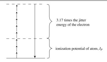
FIGURE 13.6.2: Schematic representation of the empirical relation  $\hbar\omega q_{\text{max}} = 3.17K + I_P$ . The numerical factor of 3.17 is a consequence of detailed analysis of the dynamics of an electron interacting simultaneously with an external laser field and the atomic core.
