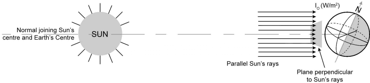
Figure 2.1: The Sun's rays incident on the Earth. I_0 = irradiance on a plane perpendicular to the Sun's rays
